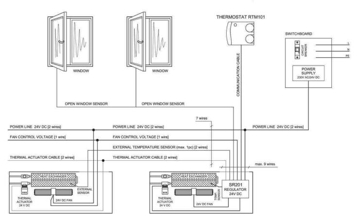
For current installation, you only need 1 thermostat, 1 regulator and 1 power supply unit per a room.
