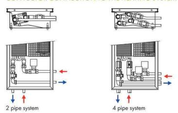
The floor convector is provided with entry holes for connection to the heating system. Connection is possible from the face side and from the side to the room.
